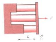
4.8 A hydraulic cylinder of 80 mm inside diameter and 4 mm wall thickness is welded to rigid end plates as shown in Fig. 4.15. The end plates are tied together by four rods of 8 mm diameter symmetrically arranged around the cylinder. Calculate the stresses in the rods and the cylinder at the cylinder design pressure of 20 MN/m². The cylinder and tie rods are made from steel with a Poisson's ratio value of 0.3.
