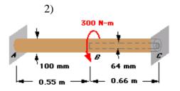
Circular shaft  $\mathcal{AE}$  has a 100-mm outside diameter. Section  $\mathcal{BE}$  of the shaft is hollow and has a wall thickness of 18 mm. A 300 N-m torque is applied as shown. We wish to determine the reactions at  $\mathcal{A}$  and  $\mathcal{E}$ . The shear modulus for this material is 80 MPa.
