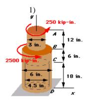
The vertical shaft shown is attached to a fixed base at  $\mathcal{D}$ . A 4.5-in.-diameter hole has been bored into section  $\mathcal{ED}$ . Determine the angle of twist at  $\mathcal{A}$  if the material is steel with  $\mathcal{E}=12\times10^6$  psi.
