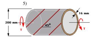
A pipe is formed by bending a 16-mm-thick plate and butt welding the plate along a helix forming an angle of 45° with the horizontal. Determine the maximum torque that can be applied if the allowable normal stress along the helix is 85 MPa.
