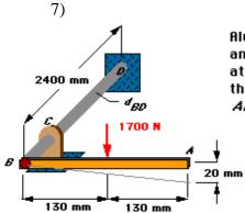
Aluminum shaft BCD(G = 70 GPa) is fixed to a wall at D and a rigid bar at B and passes through a smooth bearing at C. Determine the required diameter of shaft BCD so that when a 1700-N load is applied as shown, end A of bar AB does not deflect more than 20-mm.
