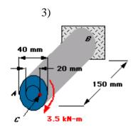
A 3.5 kN-m torque is applied to a solid cylindrical aluminum shaft. Determine the maximum shearing stress in the shaft and the percent of the torque carried by the portion of the cylinder within the 10-mm radius.
