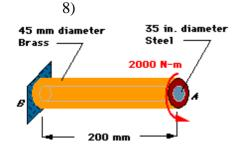
A bimetallic shaft with a 35-mm-diameter solid steel core and 45-mm-outside-diameter brass casing is loaded and supported as shown. Determine the maximum shearing stress in the steel core and brass casing knowing  $\mathcal{B}_{\rm br}$  = 39 GPa and  $\mathcal{B}_{\rm st}$  = 80 GPa.
