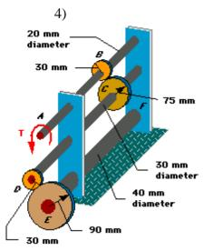
Each shaft of the gear train shown has an allowable shearing stress of 65 MPa. Determine the largest torque T that may be applied at 4.
