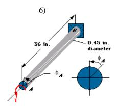
A solid steel shaft is subjected to an end torque T. The yield stress of the material in shear is 30 ksi. Knowing that for this material  $\mathcal{E}=11.5\times10^6$  psi, determine the angle of twist (in degrees) of end  $\mathcal{A}$  when yielding occurs.
