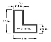
A hollow section has the shape and dimensions shown. The thickness of the section is 0.15 in. Knowing that the maximum shearing stress may not exceed 10 ksi, determine the maximum allowable torque that may be applied.
