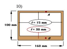
A hollow section having the shape and dimensions shown is subjected to a 2000 N-m torque. Determine the shearing stress at points  $\mathcal A$  and  $\mathcal B$ .
