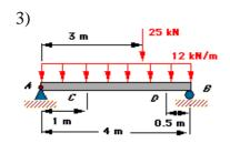
Beam AB is subjected to a uniformly distributed 12-kN/m load and a concentrated 25-kN force. Determine the deflection of the beam at points  $\mathcal L$  and  $\mathcal D$ , knowing that
