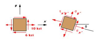
For the state of plane stress shown, determine the range of angles  $\boldsymbol{\theta}$  for which
