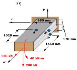
The 340  $\times$  680-mm cantilevered beam shown is subjected to the loads indicated. Determine the principal stresses and the principal angle at point  $\mathcal A$  or  $\mathcal B$  or  $\mathcal E$ . Click on the point you wish to consider. Click the exit arrow to exit this quiz.
