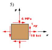
Determine the magnitude of the shearing stress that can be sustained by this element so that the maximum principal stress does not exceed 24 ksi.
