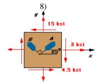
The state of stress at a point in a structural member is as shown. Two strain gages are applied to the surface of the member. The orientation of gage  ${\cal A}$  is as shown. Strain gage  ${\cal B}$  is perpendicular to gage  ${\cal A}$ . Knowing that for this material  ${\cal E}=10\times10^6$  psi and  ${\cal V}=0.33$ , use Mohr's circle to determine the strain in gages  ${\cal A}$  and  ${\cal B}$ .
