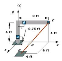
The uniform 3.5-in.-radius bracket shown is fixed to the ground at  $\mathcal{E}$ . Cable  $\mathcal{E}\mathcal{D}$  has a tensile force of 4 kip produced by turnbuckle  $\mathcal{E}$ . Determine the principal stresses and the principal angle at point  $\mathcal{A}$  or  $\mathcal{B}$ . Click on the point you wish to consider.
