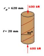
A closed-end pressure vessel has an inside diameter of 1200 mm and a wall thickness of 20 mm. It is pressurized to an internal pressure of 5 MPa and has a centric compressive force of 600 kN applied as shown. The tank is welded together along a helix making an angle of 40° to the horizontal. Determine the normal and shearing stresses along the helix.
