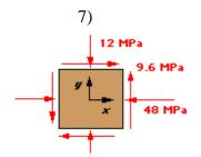
The state of stress at a point in a structural member is determined to be as shown. Knowing that for this material  ${\it E}$  = 200 GPa and  ${\it V}$  = 0.3, use Mohr's circle to determine the principal strains and the principal angle associated with this state of stress.
