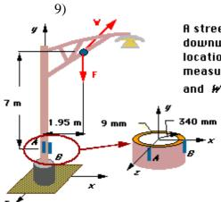
A street light with  $\it E$ = 70 GPa and  $\it V$ = 0.33 is subjected to a downward force ( $\it F$ ) and a wind load ( $\it H'$ ) as shown. At the location indicated, two strain gages are applied so that they measure the strain in the  $\it y$  direction. Determine the loads  $\it F$  and  $\it H'$  knowing that  $\it E_{\it A}$ = 350  $\it \mu$  and  $\it E_{\it B}$  = -26  $\it \mu$ .
