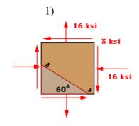
The state of stress at a point in a structural member is determined to be as shown. Using transformation equations, determine the normal and shearing stresses acting on plane a-a.
