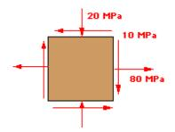
The state of stress at a point in a structural member is determined to be as shown. Using the appropriate equations, determine the maximum and minimum normal stresses, principal angle, and maximum in-plane shear stress at this point.
